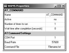
The AT Command test lets you send a text file containing valid AT phone control commands to the attached phone
